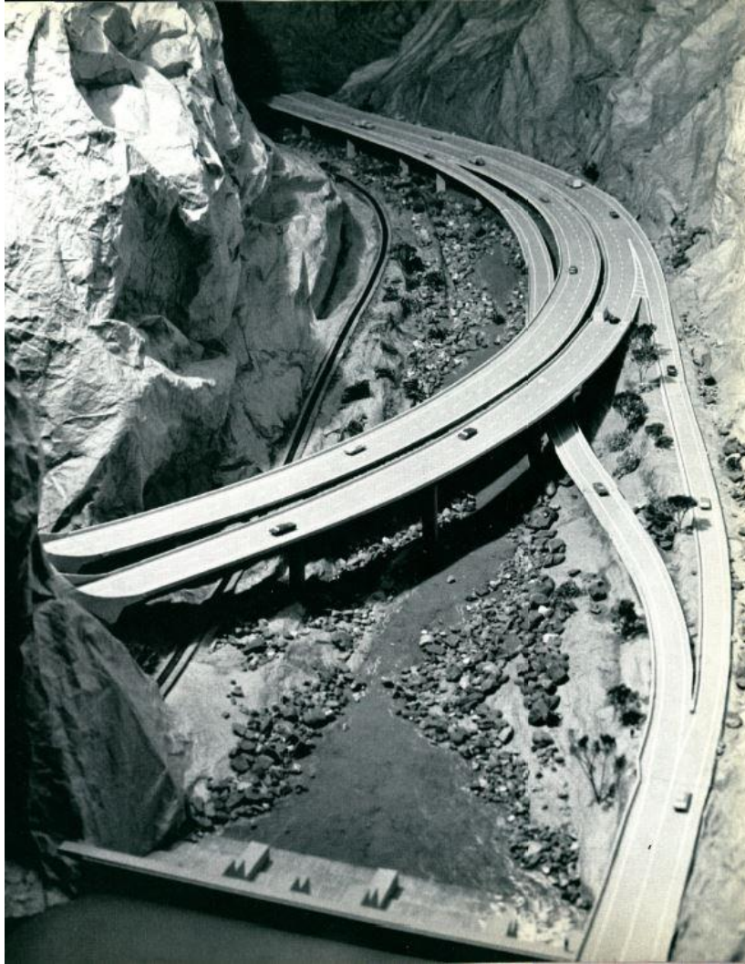
Figure 7. Photograph of a model created for the highway at Hanging Lake to illustrate and analyze the visual impact of the highway. This model exemplifies the dilemma faced by engineers and designers: fitting a four-lane Interstate Highway with on- and off-ramps into a narrow canyon with minimal impacts to the ecology of the Colorado River and Glenwood Canyon. 64
